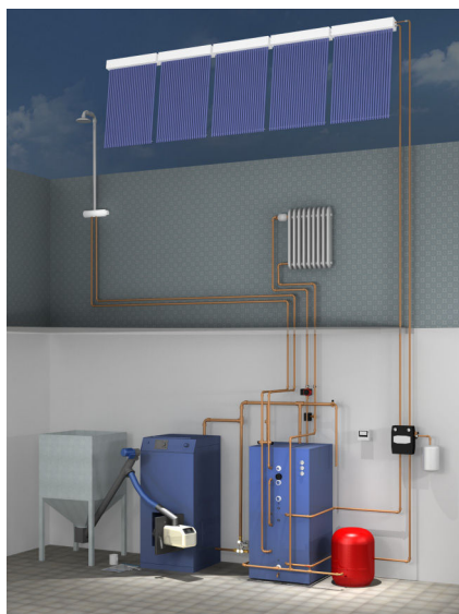
Figure 3. An example of a pellet boiler with a solar heating system. This system can easily provide space heating and hot water all year round. Illustration: Baxi
